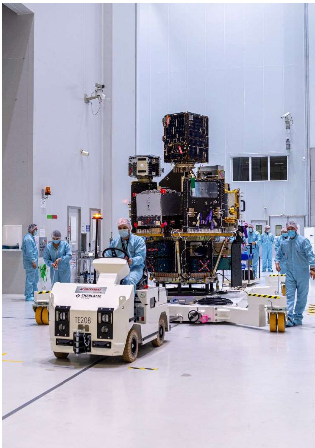
Transfer of the Small Spacecraft Mission Service (SSMS) dispenser with all satellites mounted at Europe's Spaceport © ESA
